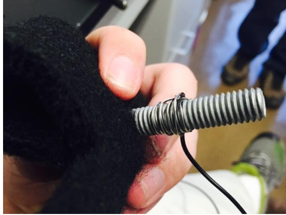
Figure 6: Aluminum Wire Wrapped Around Bolt
