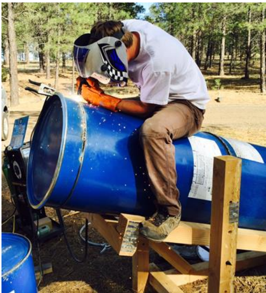
Figure 10: Welding the Drums Together and the Valves on the Top of the Digester
