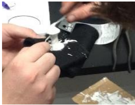
Figure 7: Epoxy Coating the Screw
